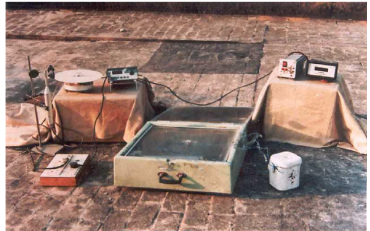
Fig.3. Experimental arrangement for determination of F_1 and F_2
